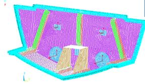
Displacement of nodes has been prohibited in all directions (UX, UY, UZ). Rotation is allowed.
