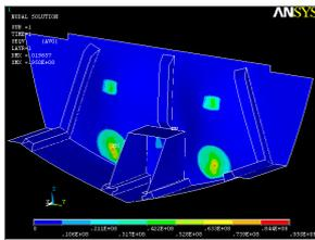
LAYER 2: Transom, Bracket, Connections – 0/90 Glass knitted rowing; Stiffener sides, Stiffener heads – Glass/Carbon Hybrid rowing
